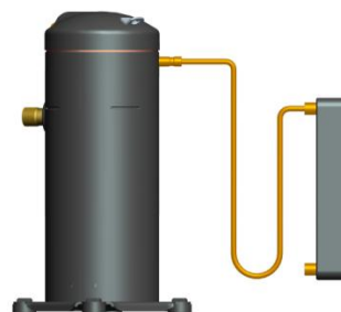
Figure 5(a) Typical line arrangement
