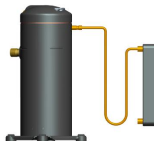
Figure 5(a) Typical line arrangement
